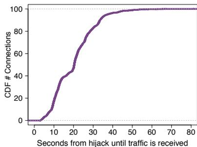
Fig. 6: Intercepting Bitcoin traffic using BGP hijack is fast and effective: all the traffic was flowing through the attacker within 90 seconds. Results computed while performing an *actual* BGP hijack against our own Bitcoin nodes.
