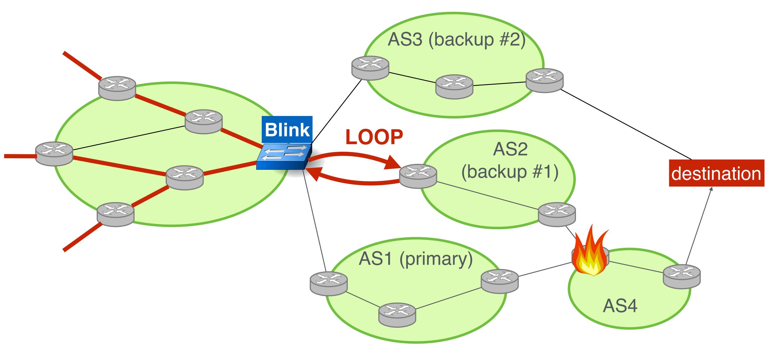
Solution: As for failures, *Blink* uses data-plane signals to pick a working backup path
