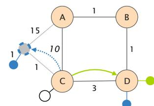
Figure 3: Fibbing in action. By injecting a fake node between A and C pointing to A, Fibbing manages to divert the blue traffic (and nothing else) upwards.
